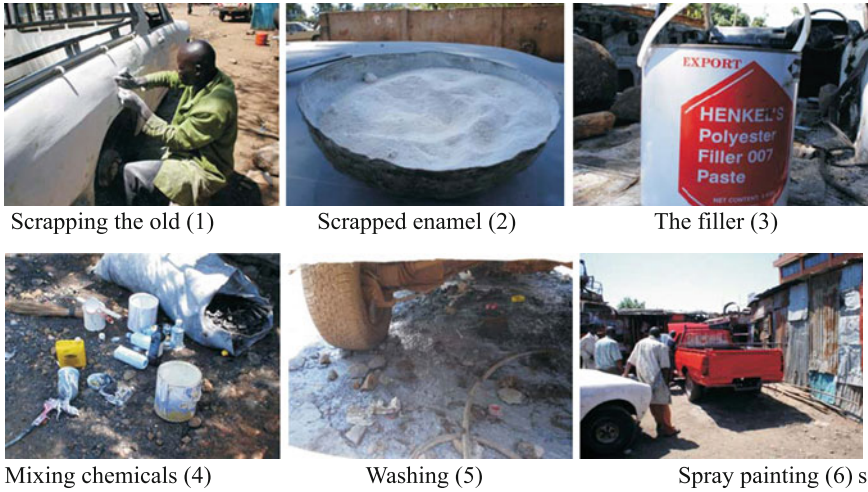
Fig. 27.8 The spray painting process and wastes in Kisumu (Kenya)
