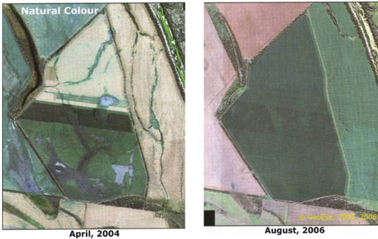
Fig. 23.8 GNSS topographical map taken by CTF overlaid on a high resolution IKONOS imagery. The left figure was taken in April 2004 (see Fig. 23.7) above. The right figure indicates the same area in August 2006 after drainage was undertaken in 2005. Source http://www.ctfsolutions.com.au
