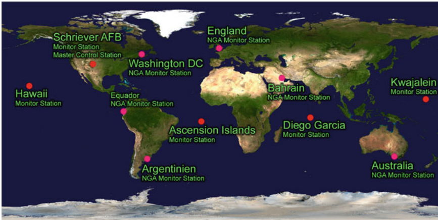
Fig. 5.2 GPS monitoring stations. Source http://www.kowoma.de/en/gps/control_segment.htm
