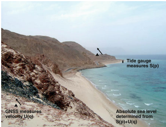
Fig. 26.12 GNSS absolute sea level monitoring. Source Awange (2012)
