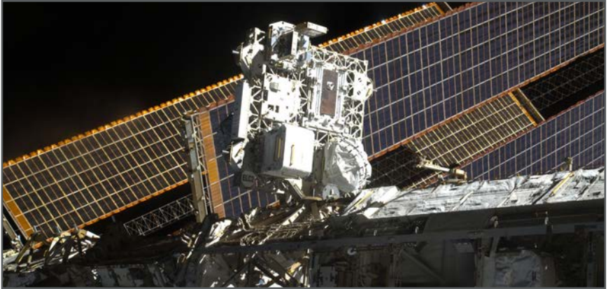
Figure 17 a. Materials International Space Station Experiment-7 on EXPRESS Logistics Carrier 2, Site 3 shortly after deployment during STS-129 in November 2009.
