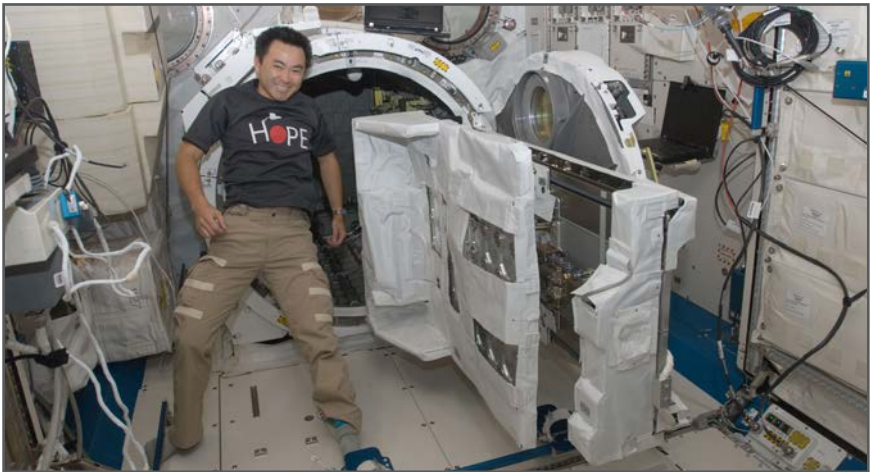
Figure 14. Multi-Purpose Experiment Platform installed on the Japanese Experiment Module Slide Table.
