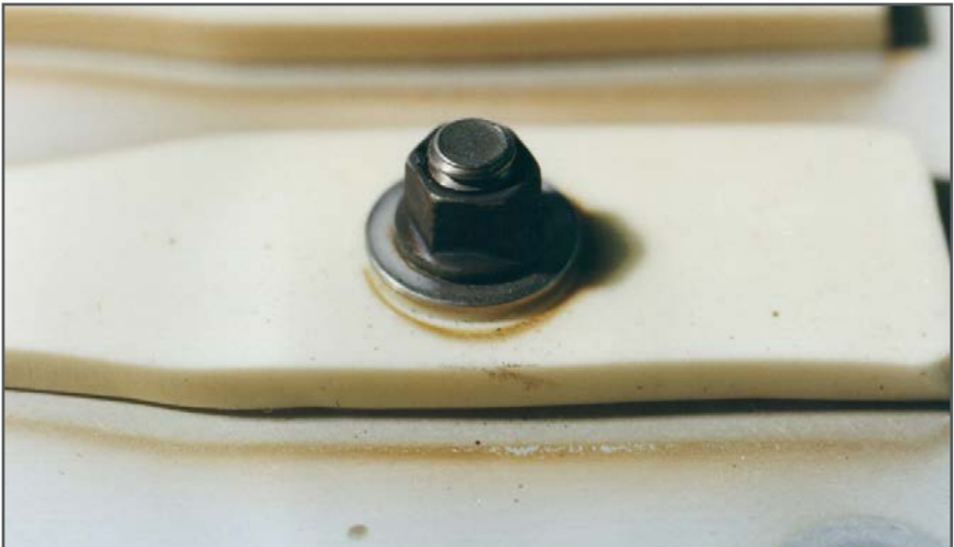
Figure 9. Postflight photograph shows a room temperature vulcanization sample from the Long Duration Exposure Facility A0171 experiment with deposited silicone contaminant on baseplate and sample. Also note oxidized silver fastener.
