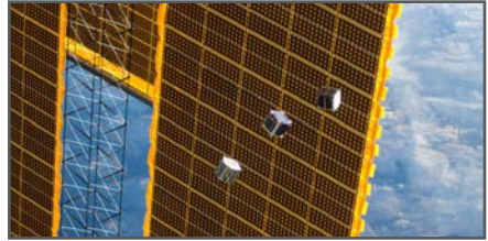
Figure 16. CubeSats deployed from the J-SSOD and photographed against an ISS solar array background.
