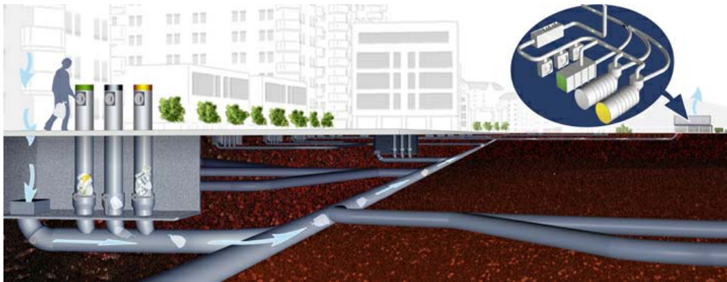
Figure 8.3 The AVAC system (Source http://www.envacgroup.com/ )
